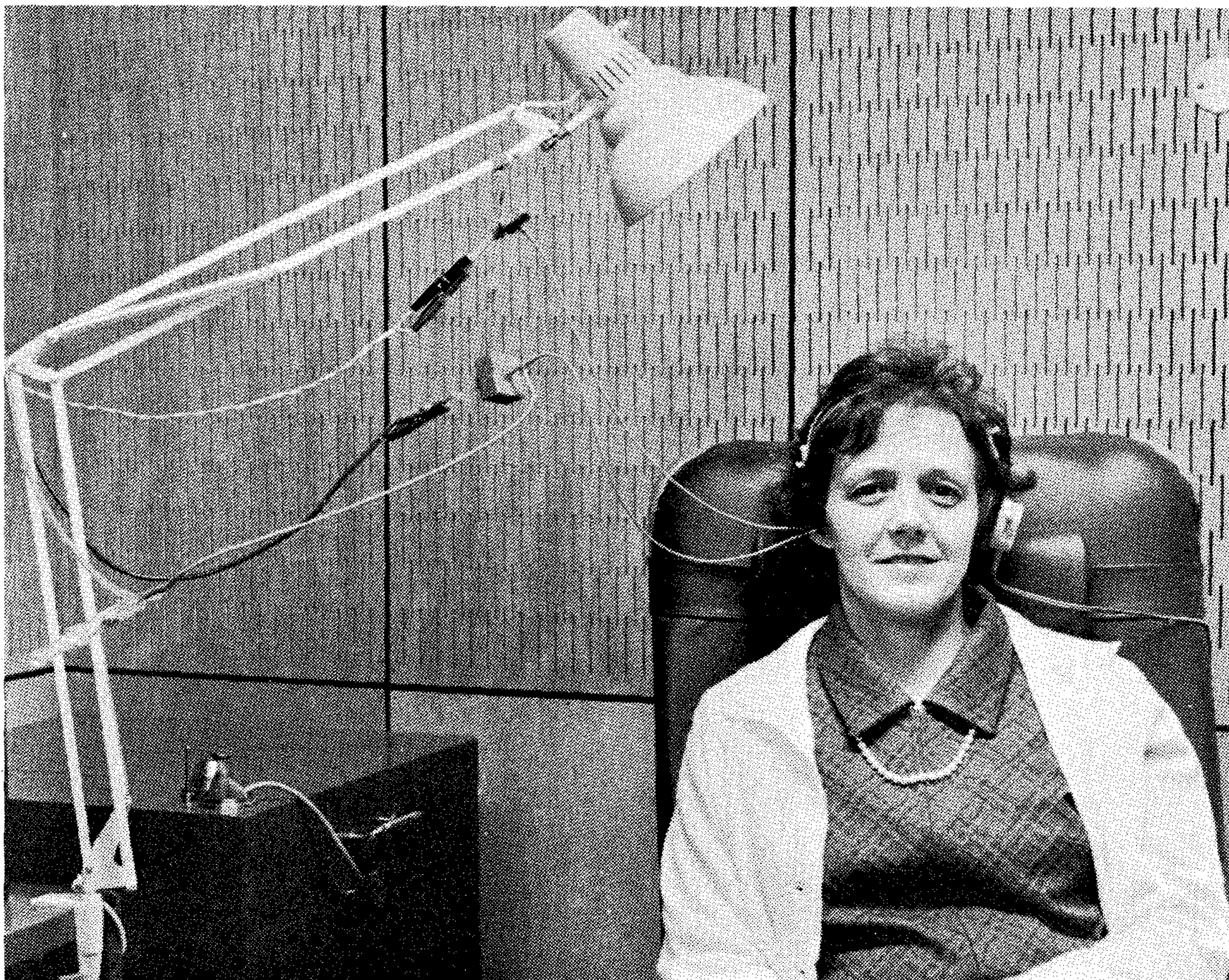
Fig.3. A patient prepared for impedance testing. Note the air-tight system suspended from the angle-poise lamp.
